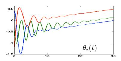
coupling large &  $|\omega_i - \omega_j|$  small  $\Rightarrow$  coherence & frequency sync
