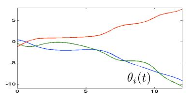
coupling small &  $|\omega_i - \omega_j|$  large  $\Rightarrow$  incoherence & no sync
